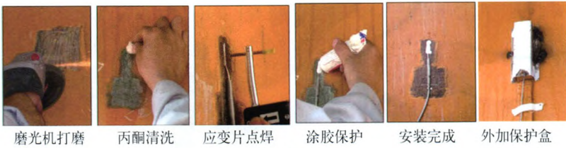
图7 应变测点布置
