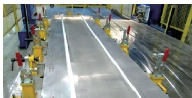
(c) FSW枕梁焊接示意
