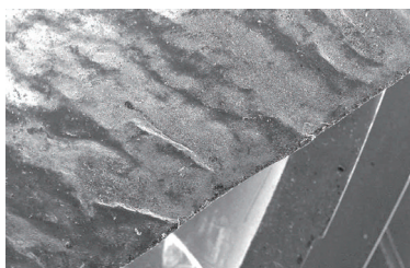
(a) 扫描电镜下裂纹形态 (2mm)
