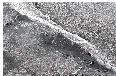
(b) 扫描电镜下裂纹形态 (500 μm)
