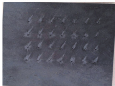
图9 激光在钢板上划线打点试验状态
