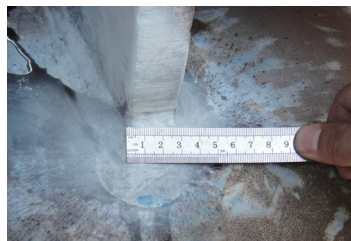
(c) 左4 (裂纹长度3 mm)
