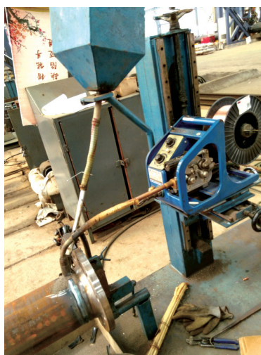
(c)外侧焊缝焊接
