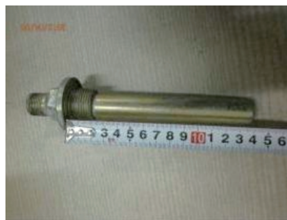
(c) 测温管插入油箱140 mm
