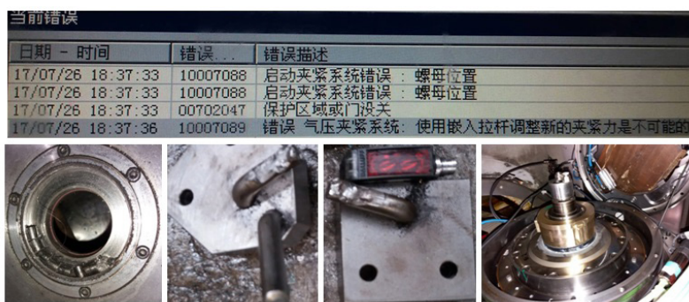
图5 Oerlikon C50切齿机B轴夹紧系统故障
