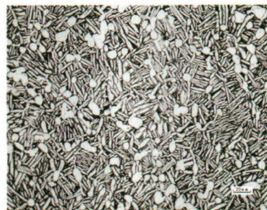
(a) 1-1 ( T_{\beta}-10^{\circ}\text{C} 锻造, T_{\beta}-30^{\circ}\text{C} 退火一热处理)
