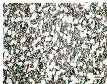
(c) 2-1 ( T_{\beta}-20^{\circ}\text{C} 锻造, T_{\beta}-30^{\circ}\text{C} 退火一热处理)
