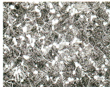
(b) 1-2 ( T_{\beta}-10^{\circ}\text{C} 锻造, T_{\beta}-50^{\circ}\text{C} 退火一热处理)
