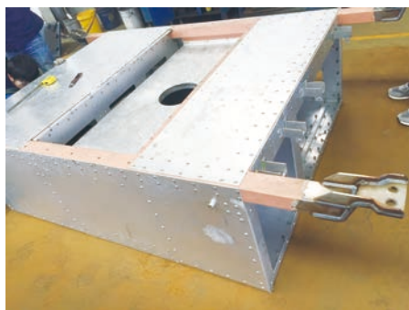
(a) 框架环槽铆钉铆接
