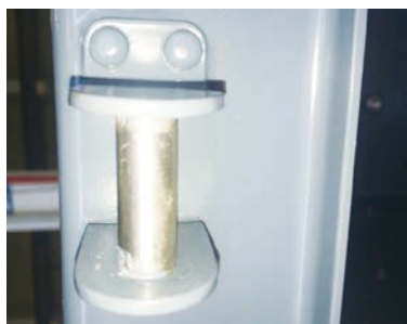
(c) 门搭扣环槽铆钉铆接
