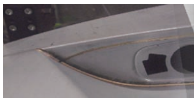
图6 GLK举升门激光钎焊焊缝
