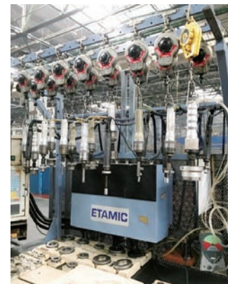
(c) 检测离合器壳总成孔径
