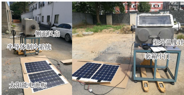
图3 全自动太阳能驱动半导体制冷系统的实物 Fig. 3 Actual photos of fully-automatically solar-energy driven refrigeration via semiconductor
