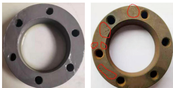
a) 1#试样低倍形貌 (切割面) b) 1#试样低倍形貌 (麻坑面)
