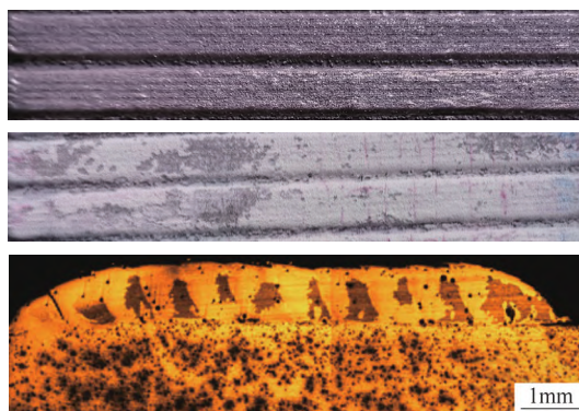
b) 涂层2激光熔覆成形和接头
