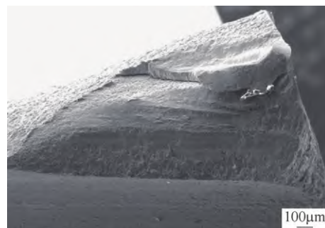
a) 线源起源SE2信号形貌 (52×)
