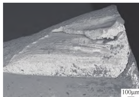
b) 线源起源BSD1信号形貌 (52×)
