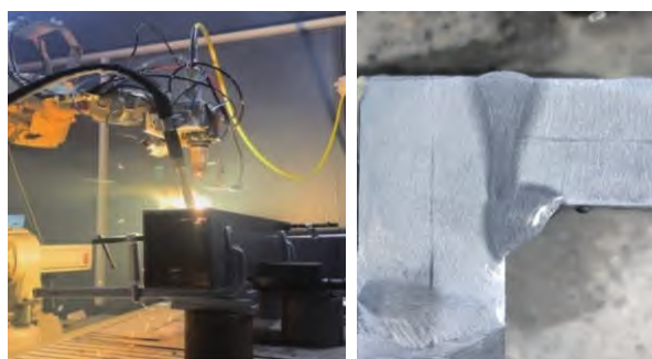
a) 箱形柱棱角焊缝激光复合焊
