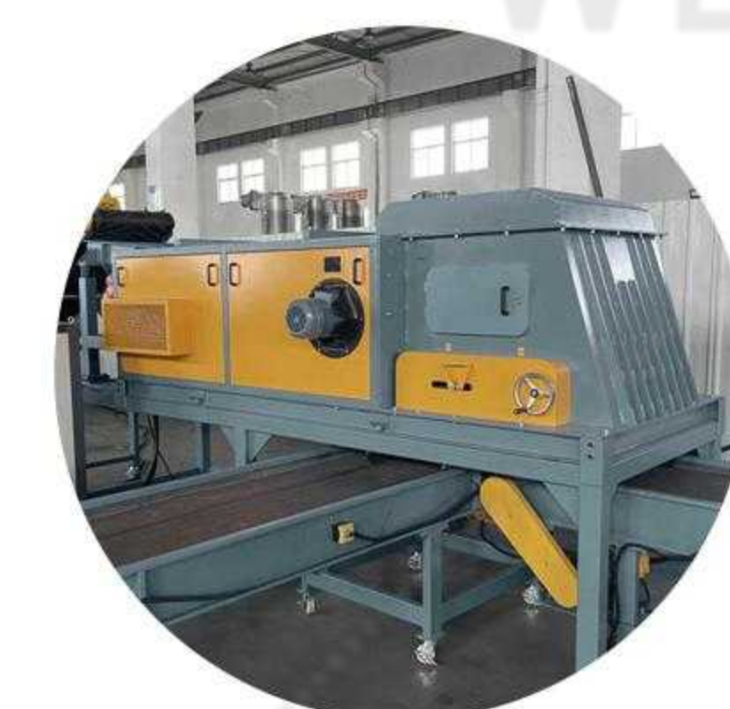
涡电流分选机 将有色金属和塑料等杂质分离 Eddy Current Separator Separate non-ferrous metals and impurities like plastics
