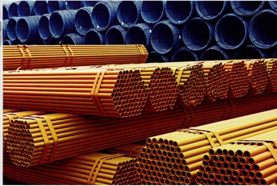
黄色防锈漆钢管 Yellow rust-proof paint steel tubes
