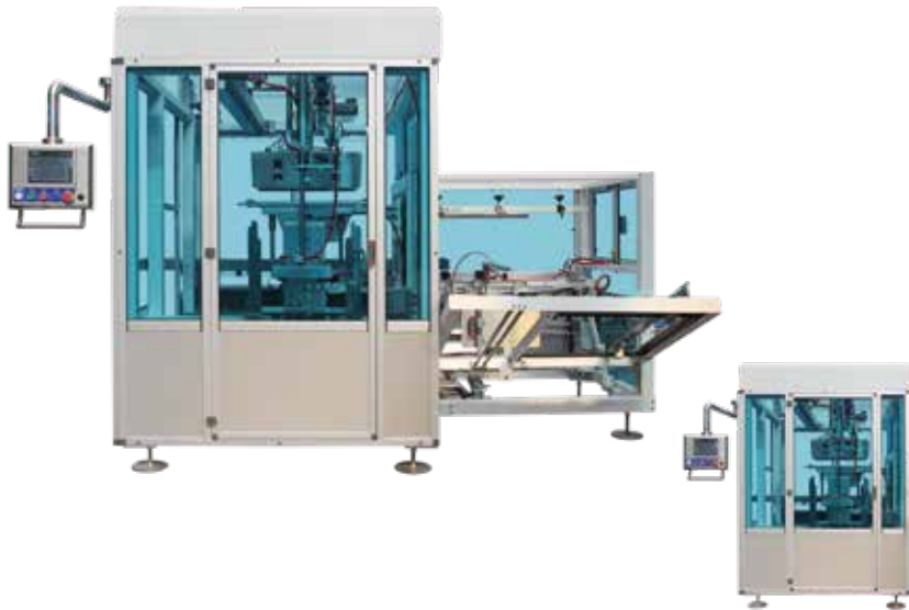
YS-CXF-J-10T 平移式装箱机 (抓手) Translational carton packer (Gripper)
