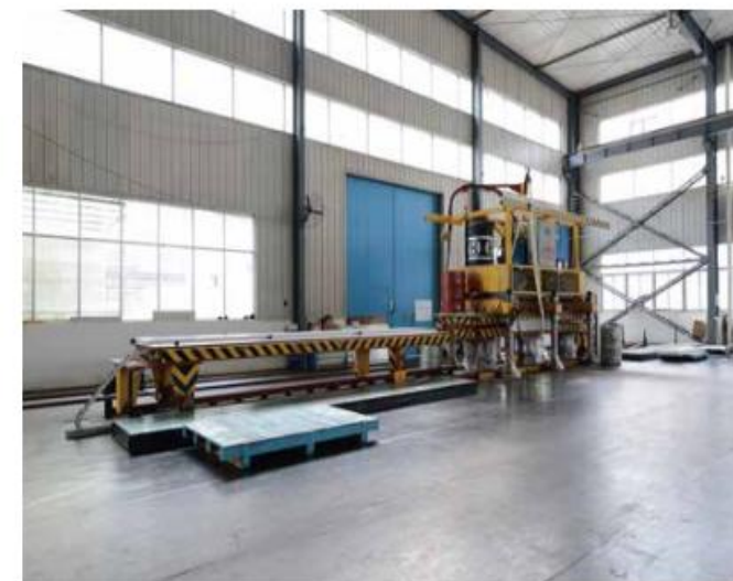
美国瑞科的聚氨酯高压喷射式发泡机组成的空调器保温面板生产线。 The production line of thermal insulation panel for air conditioner consisting of Polyurethane High Pressure Jet Foaming Machine of Rico, USA.
